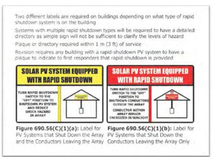
TURN RAPID SHUTDOWN SWITCH TO THE "OFF" POSITION TO SHUT DOWN PV SYSTEM AND REDUCE SHOCK HAZARD IN ARRAY.
